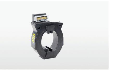
The CMV current transformer is primarily used for pad-mounted distribution transformer metering. The CMV-Hi Temp transformer is used for metering on 600 V systems inside high ambient temperature environments (85° C).
